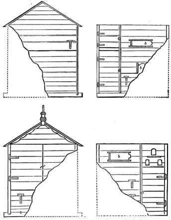
FIG. 58.-To show arrangement of Nest-boxes and Slip-doors.
