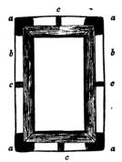
FIG. 92.—Blocks for Picture-frame fixing. a. Blocks; b. string; c. tightening wedges.
