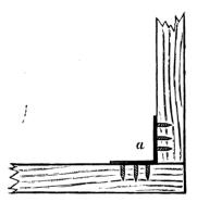
FIG. 52.-Spars joined by "angle" iron.
