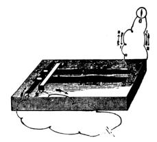
FIG. 148.—Key-board connected with battery and coil to show how the needle is moved.
