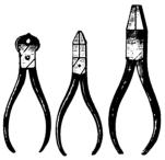
FIG. 107.-Cutting Pliers.
