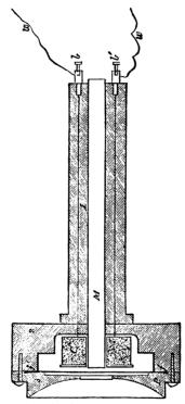
FIG. 149.—Section of the Telephone. m. The magnet; c. the bobbins of wire; f. the thin plate held by mouthpiece; b. binding-screws attached to line wires.
