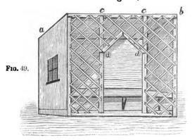
angle at which the uprights must be cut, for the top side piece to be nailed to, then nail it securely on the uprights at each end. For the front and back top rail, cut the ends, using the halving joint, Fig. 21. Put it into position, as Fig 49, b. Bore two good holes, and drive in 3-inch nails. It would be as well to char or tar the ends before putting them into the ground, as we directed for the swing.
