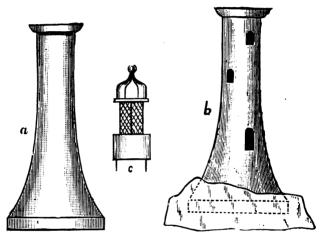
FIG. 96.—Model of Lighthouse. a. Turned block for shaft; b. shaft mounted on rock; c. lantern of Lighthouse.
