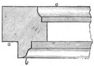
FIG. 93.—Moulding used for Frame. a. is called the rebate; b. the sight edge; c. the back or outside edge.
