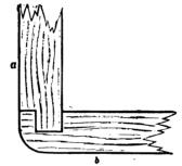
FIG. 68.—Tongued and grooved joint for small work.
