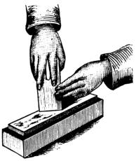
FIG. 12.-Sharpening a Plane-iron.
