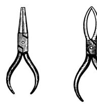
FIG. 108.-Round-nosed Pliers.
