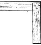
the thicker part of the square is held close to the edge, and run along the same, the small blade points out all along it a direction at right angles to that edge.
