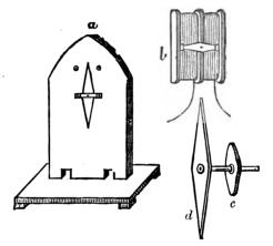
FIG. 146.—Separate parts for Needle Telegraph.
