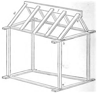
FIG. 56.—Frame-work of Out-house.
