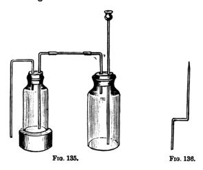
it cools, the platinum tip will be fixed tightly. A straight jet about 6 inches long attached to the end of a length of indiarubber tubing is sometimes even more convenient than that we have described.
